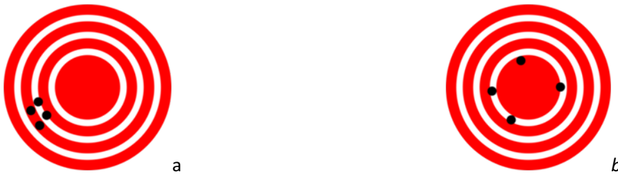
Fig.3. Illustration of systematic and statistical errors: a) low accuracy, high precision; b) high accuracy, low precision
