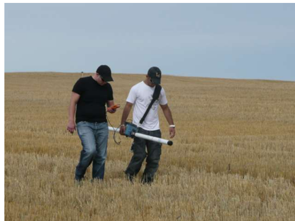
Figure 1: Principle of electromagnetic induction (EM) sounding measurements of the underground conductivity (left, Tx and Rx are the transmitter and receiver coils, respectively); Typical EM measurements with a Geonics EM31MK2 instrument (right; photo by C. Haas @ southern Alberta).
