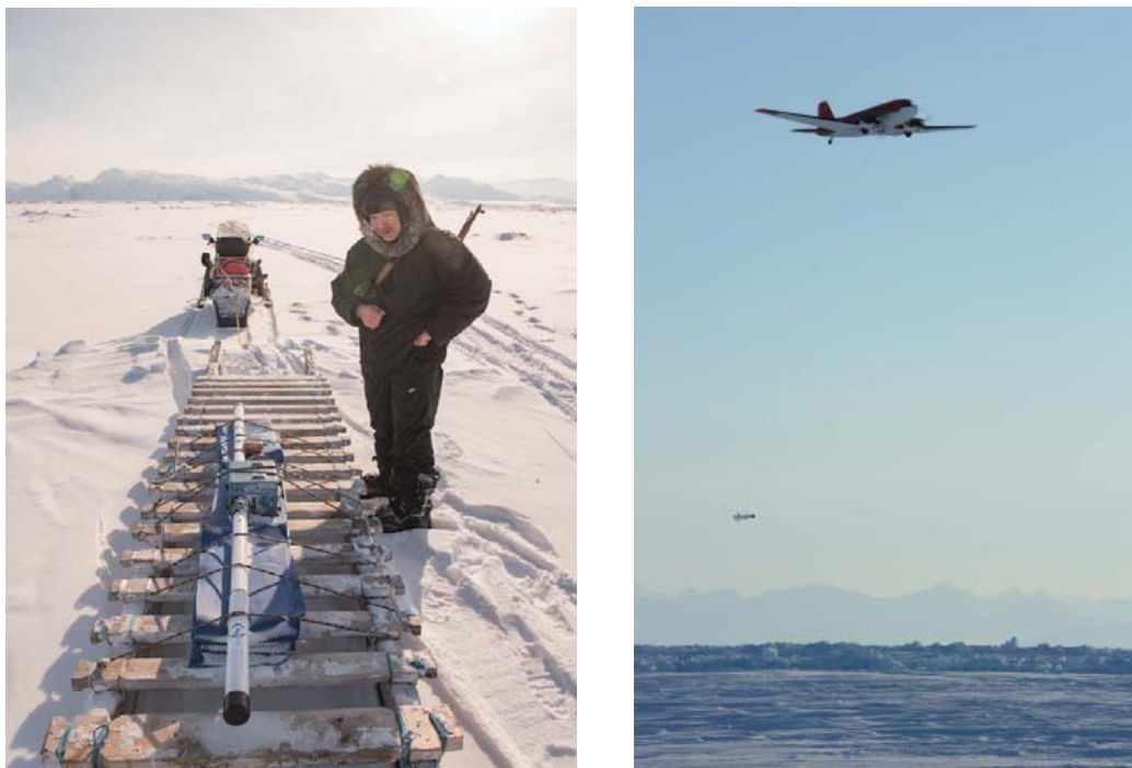
Figure 3: Examples for ice thickness measurements by snowmobile (left; compare instrument with Figure 1) or aircraft (right, using a towed EM Bird).
