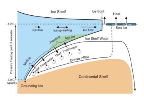
Conceptual picture of sub-ice shelf overturning, where the layer interacting with the ice shelf is assumed to be sufficiently thin that friction dominates over rotation in the force balance.
